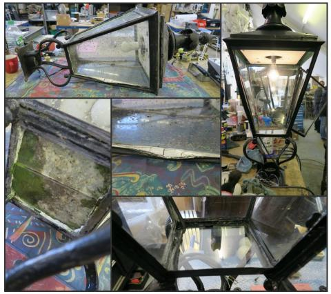
rust was removed, a fresh layer of white waterproof paint was added to the inside. The pair were then rewired with thick waterproof electrical cable and the original / replacement glass panes sealed in to the frame, with sealant that would not expand as it had done previously and damaged the metalwork. The lanterns were finished with one of our dimmable 7w GLS bulbs which should give of plenty of light during the dark winter nights!
